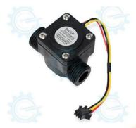
SEN-HZ21WA flow sensor can be used to accurately measure liquid volume and rate of flow flowing through it. It output digital pulses at frequency in proportion to the rate of flow. Accumulated number of pulses, on the other hand, gives an accurate measure of the liquid volume. Compatible in all gizduino boards and MCUs
